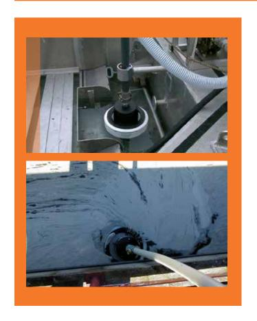
The TERRAPIN has been designed with industrial applications in mind. The unit may be used free floating with a 1½ in suction hose connected to the underside. Alternatively a suction hose, connected to the top of the skimmer, can suspend the TERRAPIN. The diameter of the TERRAPIN is only 410mm / 16in, which permits access into tight and possibly hazardous areas.
