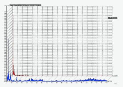
The "Y-axis" shows the energy in the vibrations. The "X-axis" indicates e.g. the frequences of the rotating elements. The vibration measurements on the pump shown were between 0.53 mm/s and 0.79 mm/s.
