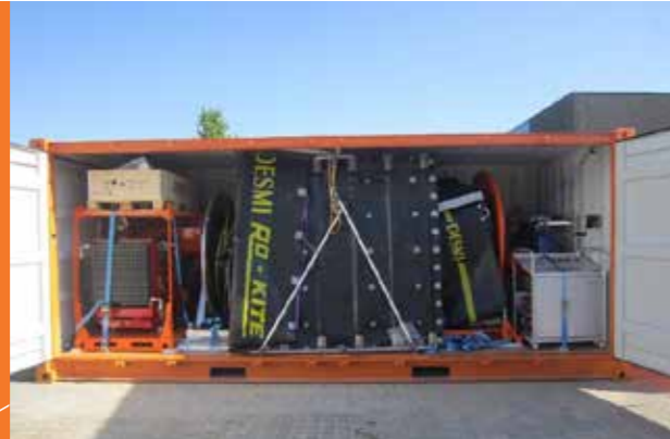
Containerized Ro-Kite 2000 with a Ultimate Speed-Sweep system
