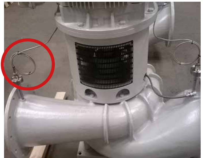
The aggressive fluid will not damage the manometers thanks to the fitted membranes.
