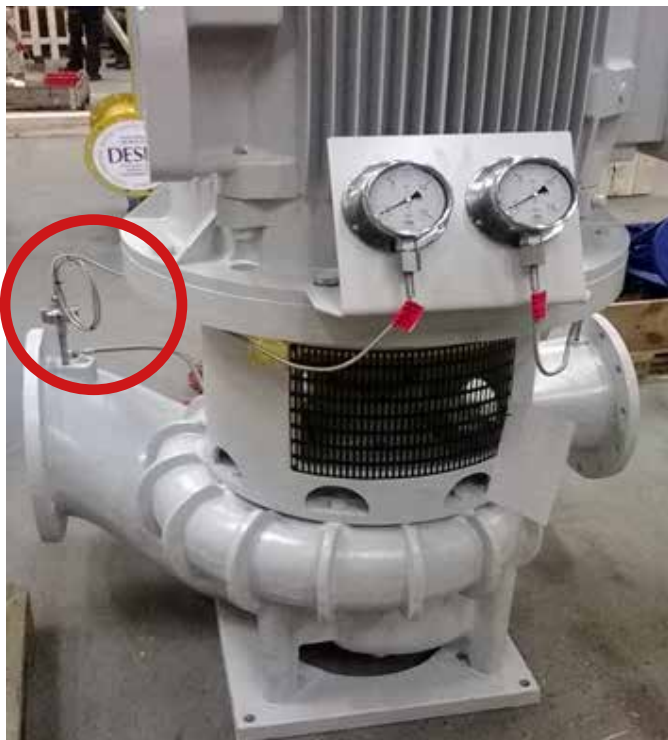
Super Duplex NSL stainless steel pump for aggressive fluids.
