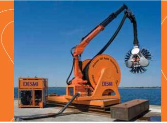
The DESMI Giant Octopus Offshore Recovery Systems are a significant step forward in design and proven technology. It is part of the recent DESMI drive of innovations over the last 18 months that include Single Point Inflation (SPI) boom through the reel, a speed sweeping system using the Ro-Boom containment boom, Ready For Dispatch systems, (RFDs) and the Arctic Range designs.
