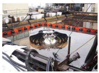
There are two, integral but removable, DESMI DOP 250 Dual pumps each with a capacity of  $125\text{m}^3/\text{h}$  / 550 gpm giving a total of  $250\text{m}^3/\text{h}$  / 1101 gpm. The brush capacity is  $3 \times 132.6 \, \text{m}^3/\text{h}$  /  $584 \, \text{gpm}$  –  $397 \, \text{m}^3/\text{h}$  /  $1748 \, \text{gpm}$  (DNV Certified).
