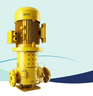
The TSL pumps are two-stage, single-suction centrifugal pumps with high differential pressure pumps including a flow up to  $48 \text{ m}^3/\text{h}$  and pressure up to 135 mLC at 60 Hz.
