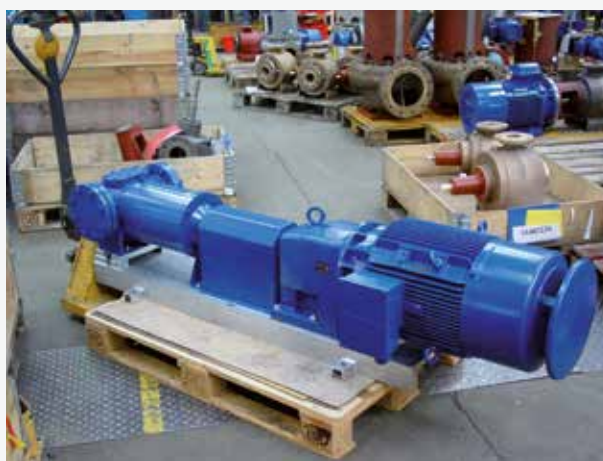
One of the magnetically coupled pumps which are used in the polyurethanes production industry.
