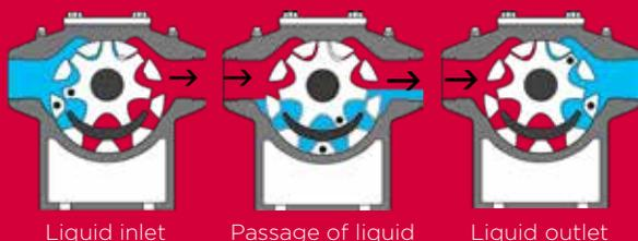
This means that superior self-priming capability and gentle liquid handling are achieved, and also that highly viscous liquids can be pumped. ROTAN® pumps offer the following additional advantages:
