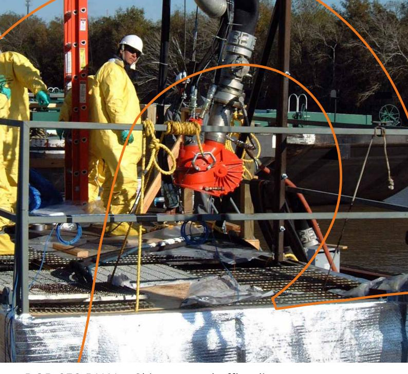
DOP-250 DUAL - Skimmer and offloading pump PROVEN OIL SPILL TECHNOLOGY
