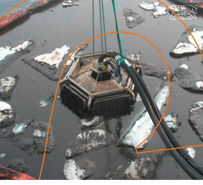
POLAR BEAR - ICE SKIMMER - New Generation of Ice Skimmers developed in cooperation with SINTEF Material and Chemistry in Norway.
