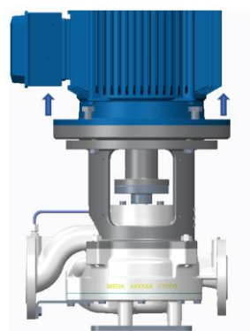
3. Loose set screws (42) ; Remove motor
