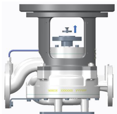
4. Loose Allen screw(36) ;Remove thrust plate(35)
