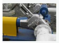
One of the ROTAN<sup>®</sup> features specifically appreciated is the simplicity of design. The pumps perform equally well in either direction.
