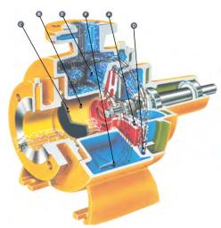
If for some reason, air penetrates into the suction pipe and the pump stops pumping, the priming process starts again as described above, and continues until normal pumping has been resumed
