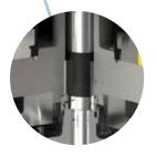
Bearings in tungsten carbide possess excellent wear-resisting properties, effectively lubricated by the pumping medium, ensuring a long life-span.
