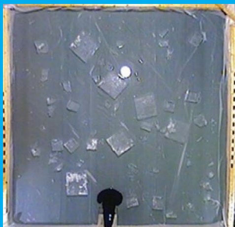
Oil is introduced into a test pan with simulated ice drift
