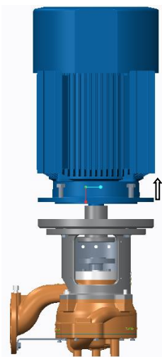
3. Loose set screws (42) ; Remove motor
