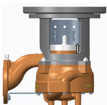
6. Loose Allen screw(25) ;Remove seal cover (28)
