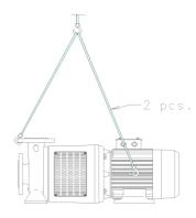
Before shipment the pump is to be fastened securely on pallets or the like. The pump is to be lifted in the following way:
