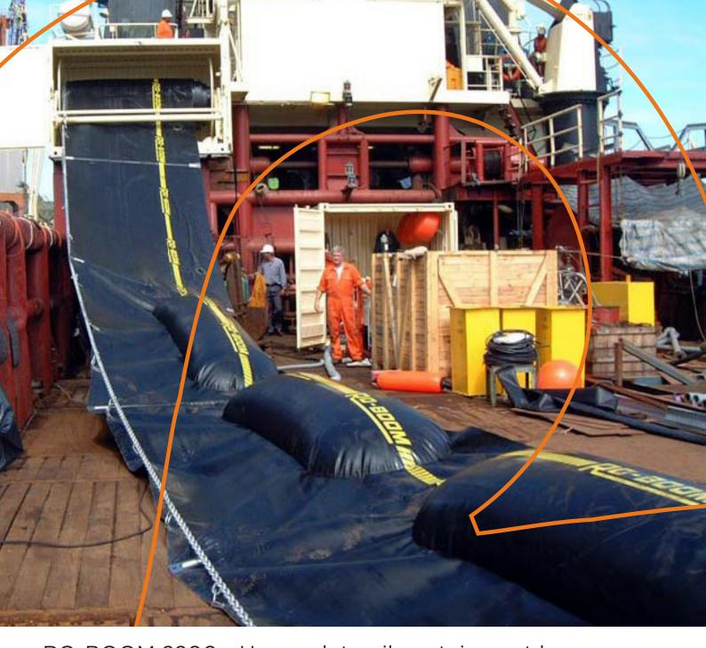
RO-BOOM 2200 - Heavy-duty oil containment boom PROVEN OIL SPILL TECHNOLOGY
