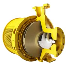
DESMI inducers are applied with variable pitch to realize a higher specific suction speed in a limited axial space. After CFD simulation and optimization, cavitation on impeller is supressed significantly with much less bubbles developed after DESMI inducers are mounted.
