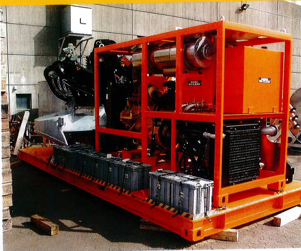
The 183-kW (245 hp) 6.8L engine drives two hydraulic piston pumps with a maximum hydraulic flow of 400 liters (106 gallons) per minute and a pressure of up to 210 bar.
