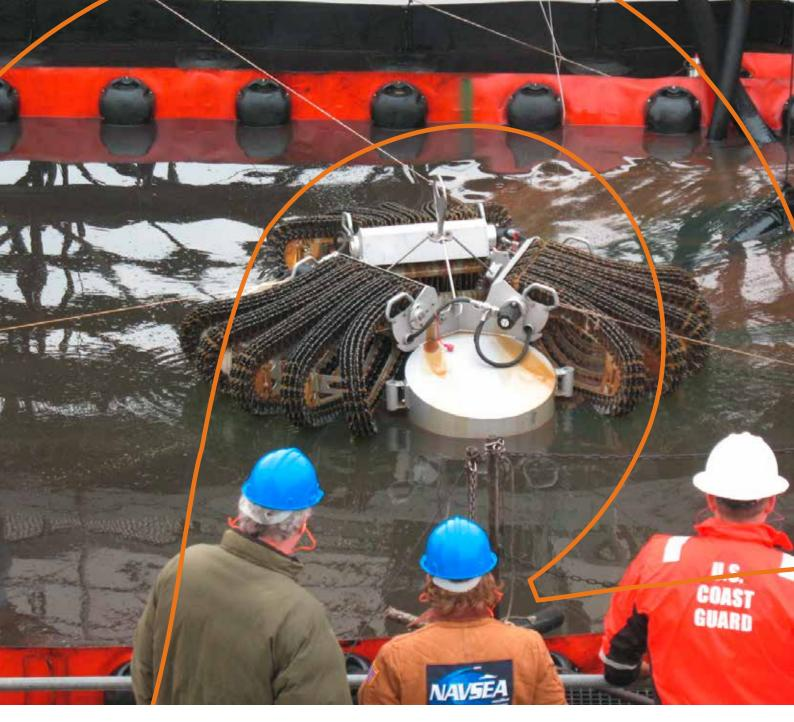
GIANT OCTOPUS - Revolutionary high capacity belt/brush skimmer PROVEN OIL SPILL TECHNOLOGY
