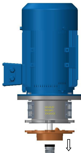
4. Remove shaft seal (22) and rear cover (4)
