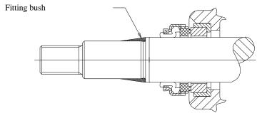
If the carbon ring is not fixed, it is important to check that it is fitted correctly, i.e. the chamfered/lapped side is to face the seat. The carbon ring can be held by a little grease. When using oil on the shaft, the bellows will settle and seat in about 15 minutes, and until then tightness should not be expected.
