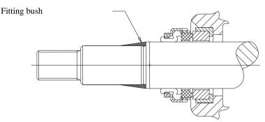
If the carbon ring is not fixed, it is important to check that it is fitted correctly, i.e. the chamfered/lapped side is to face the seat. The carbon ring can be held by a little grease. When using oil on the shaft, the bellows will settle and seat in about 15 minutes, and until then tightness should not be expected. After start, check by viewing the leak hole that there are no leaks.
