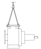
The lifting straps must not bear against sharp edges and corners.
