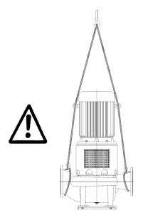
The lifting straps must not bear against sharp edges and corners
