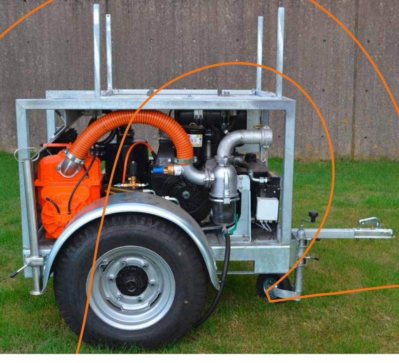
RO-VAC MKIII – The new generation of vacuum recovery system for oils and other liquids
