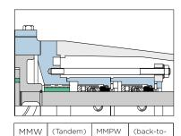
Double mechanical shaft seals, DIN 24960/EN 12756 - KU, in tandem or back-to-back, with productlubricated main bearing. Used where no leakage is allowed. Up to 16 bar differential pressure.
