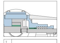
Special clearances. Increase of tolerances used for liquids with viscosities above 7,500 cSt. or temperatures above 150°C.
