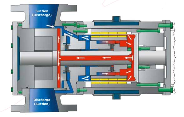
One of the distinguished features of the ROTAN<sup>®</sup> ED range is that the pumped medium is hermetically contained in the system since the magnetic coupling eliminates the need for a shaft and mechanical seal, which could allow gaseous exchange between the pumped medium and the atmosphere.
