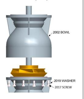
3. Loosen the allen screw (2012) and remove the lock ring (2009) and impeller (2001)
