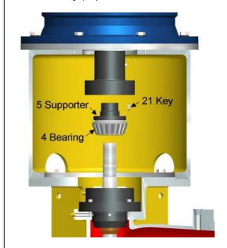
8. Loosen the allen screw (20) and take off the bearing house (3)
