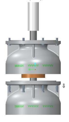
4. Loosen the Allen screw (2014) and remove the lock ring (2009) and second impeller (2001)
