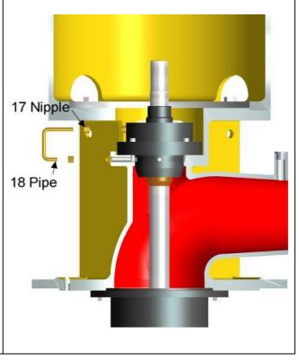
7. Pull out the bearing supporter (5) with bearing (4) along the shaft, and remove the key (21)
