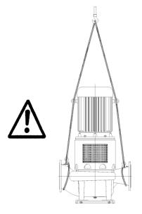
The lifting straps must not bear against sharp edges and corners
