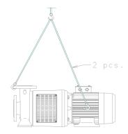
Before shipment the pump is to be fastened securely on pallets or the like. The pump is to be lifted in the following way:
