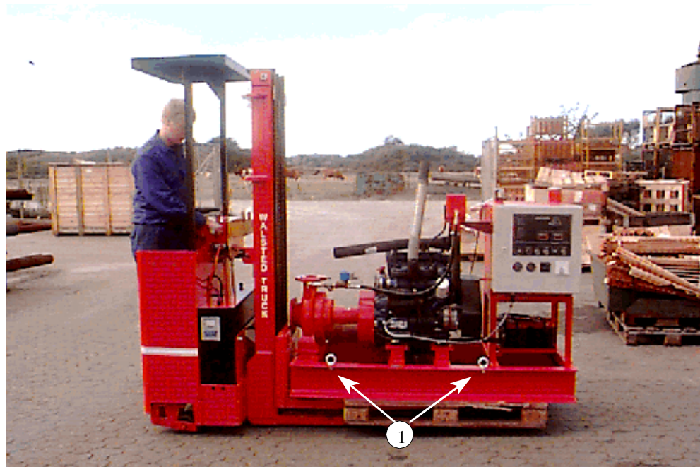
Figure 1: Transportation of sprinkler system, 1) Lifting eyes
