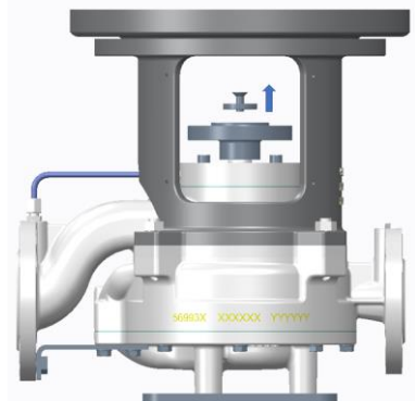
4. Loose Allen screw(36) ;Remove thrust plate(35)
