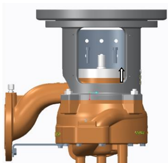
6. Loose Allen screw(25) ;Remove seal cover (28)
