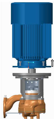
3. Loose set screws (42) ; Remove motor
