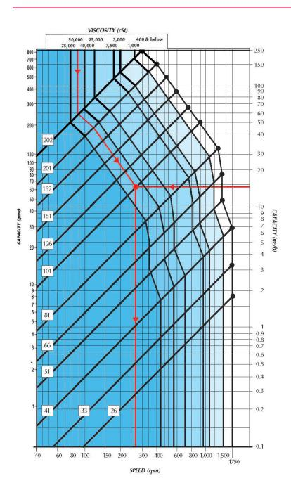
PLEASE NOTE! ED: Capacity curve up to pump size 151 GP: Capacity curve up to pump size 101
