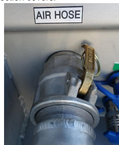
Connect the 4" Air Hose to the Control Stand
