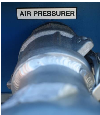
Connect the 4" Air Hose to the pressure side On the Container Bulkhead.
