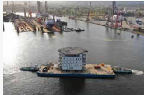
Cargo Pontoon TRD-HORIZON is equipped with 4x150 m 3 DESMI ballast pumps. The system is fully internal and can be powered from a shore connection, or optionally with a power generator
